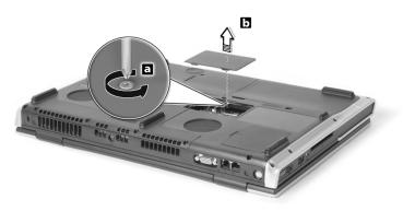
3 Insert the memory module diagonally in the slot (a), and then press down gently until it clicks in place (b).
